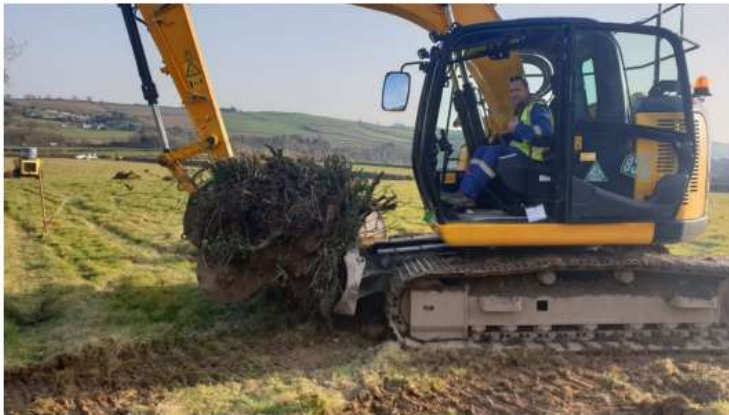
Plate 7: Small section of hedge being translocated via excavator
